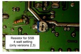
The left potentiometer is for SSB only, the right for FM (AM is automatically set to 25 % of FM power) Both potentiometers are for output adjusting in the EN 300 433 version. The maximum tunable power value is around 10 watts.
